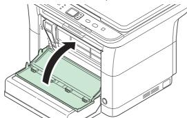
**Note** If the front cover does not close, check that the new toner container is installed correctly (in step 4).
